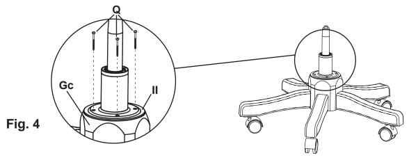
**4.** Insert the Gas Cylinder (II) into the Pedestal Assembly (Gc). The lip on the Cylinder may not sit flush against the top of the Pedestal. With a 1/8" drill bit, drill pilot holes 3/4" deep through the holes in the gas cylinder lip and into the Pedestal. Insert four #10 x 1-1/4" Black Pan Head Screws (Q) through the Gas Cylinder and into the Pedestal and securely fasten. This will draw the lip flush against the Pedestal. See Figure 4.
