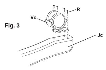
**3.** Place the Caster (Vc) over the prepunched holes in the bottom of the Foot (Jc). Screw the Caster down with four #10 x 3/4" Pan Head Screws (R). Repeat for the other three Feet. See Figure 3.
