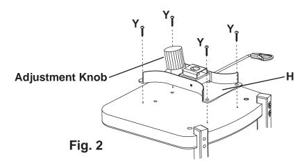
2. Turn the Tilter Mechanism (H) upside-down and place it on the bottom of the seat. Make sure the adjustment knob faces the front of the chair as shown in Figure 2. Match up the four small screw holes in the Tilter Mechanism with those in the bottom of the seat. Screw the mechanism in place with four #14 x 1" Philtruss Screws (Y).
